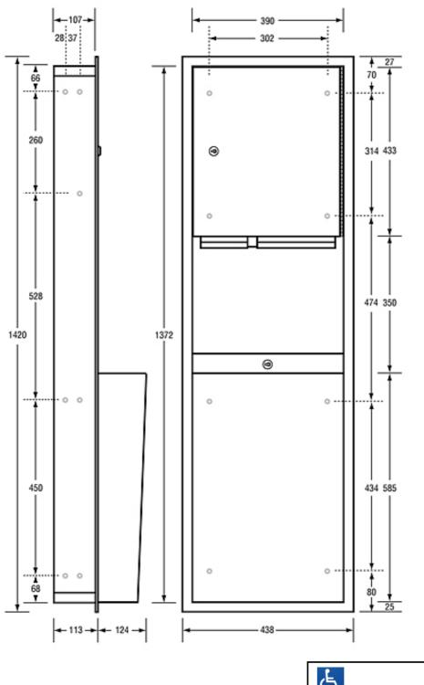
This product is AS1428.1 compliant (accessible compliant) when installed in accordance with the guidelines.
